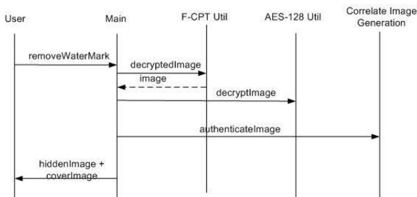
Fig. 5: Sequence flow diagram for removal of watermarking [9]
