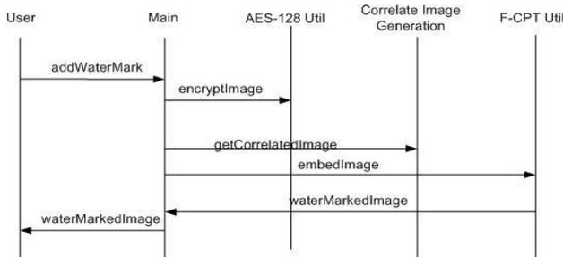
Fig. 4: Sequence flow diagram for watermarking [9]
