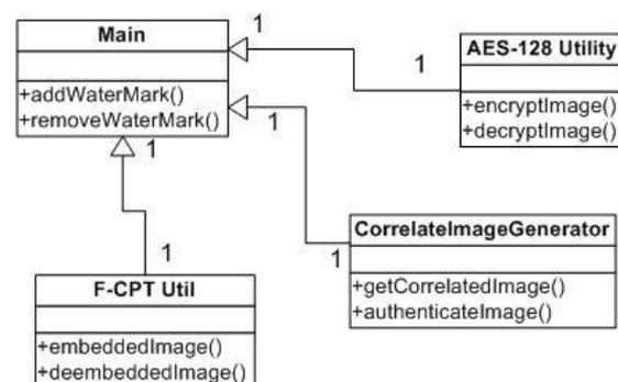
Fig. 2: Class diagram of proposed solution [7]
