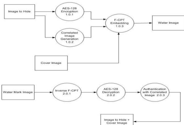
Fig. 7: Data flow diagram of level 1 of watermarking [12]
