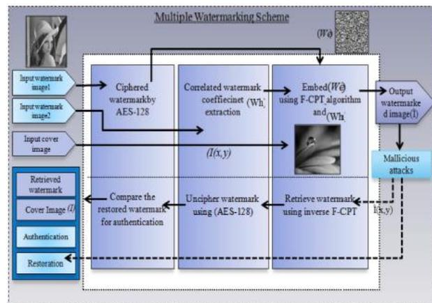
Fig. 1: System architecture of proposed solution
