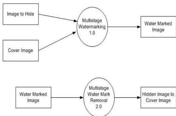
Fig. 6: Data flow diagram of level 0 of watermarking [11]
